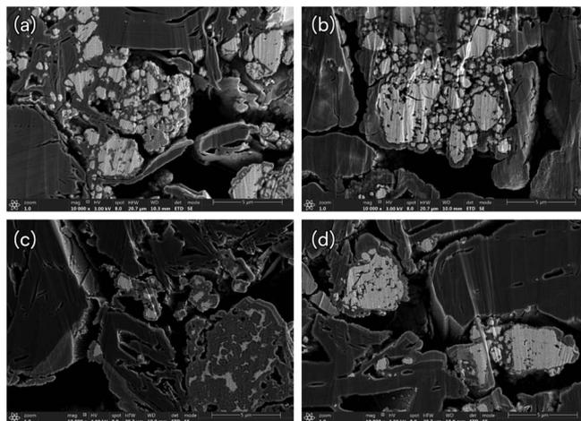
**Figure 7.** FESEM cross section images of negative electrodes from Gr:Si-alloy/LCO full pouch cells with 3EC:7EMC or 23EC:67EMC:10FEC in 1 M LiPF<sub>6</sub>. (a) Without FEC after 30 cycles, (b) with FEC after 30 cycles, (c) without FEC after 75 cycles, and (d) with FEC after 75 cycles.
