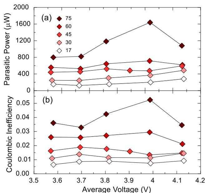
**Figure 3.** (a) Parasitic power and (b) coulombic inefficiency of Gr:Si-alloy//LCO full pouch cells with 3EC:7EMC in 1 M LiPF<sub>6</sub> electrolyte as a function of the average voltage window for various cycle numbers as indicated in the legend.
