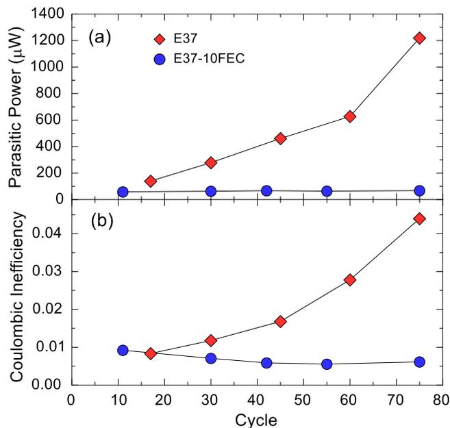
**Figure 5.** (a) Parastic power and (b) coulombic inefficiency for Gr:Si-alloy/LCO full pouch cells with 3EC:7EMC or 23EC:67EMC:10FEC in 1 M LiPF<sub>6</sub> as indicated by the legend. Values were interpolated from Figures 3 and 4 at an average voltage of 3.8 V.
