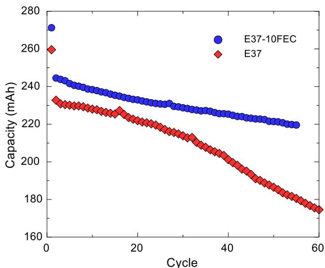
**Figure 2.** Cycle life of Gr:Si-alloy//LCO full pouch cells with 3EC:7EMC or 23EC:67EMC:10FEC in 1 M LiPF<sub>6</sub> as indicated by the legend.
