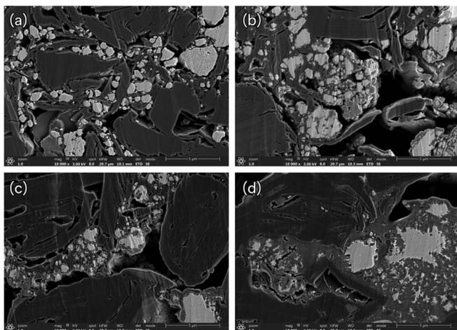
**Figure 6.** FESEM cross section images of negative electrodes from Gr:Si-alloy/LCO full pouch cells with 3EC:7EMC in 1 M LiPF<sub>6</sub>. (a) Fresh electrodes, (b) after 30 cycles, (c) after 45 cycles, and (d) after 60 cycles. Light and dark gray areas correspond to Si alloy and graphite, respectively.
