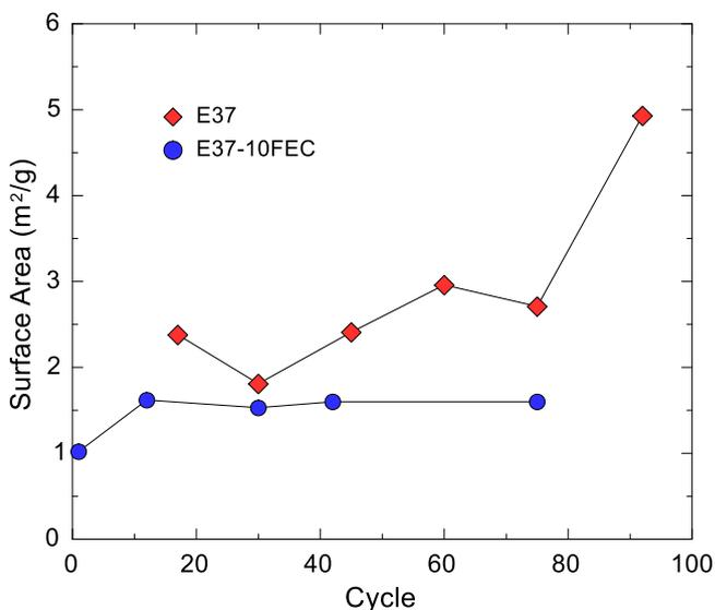
**Figure 8.** BET surface area of negative electrodes from Gr:Si-alloy/LCO full pouch cells with 3EC:7EMC (red diamonds) or 23EC:67EMC:10FEC (blue circles) in 1 M LiPF<sub>6</sub>, as a function of cycle number.
