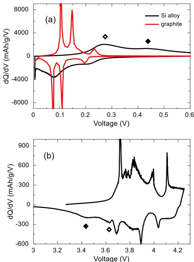
**Figure 1.** (a) Differential capacity ( $dQ/dV$  vs  $V$ ) curves of Si alloy and graphite half cells, Si alloy delithiation peaks are identified by diamonds. (b) Differential capacity curve of a Gr:Si-alloy/LCO full cell with the corresponding Si alloy delithiation peaks marked by diamonds.
