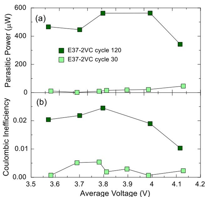
**Figure 11.** (a) Parasitic power and (b) coulombic inefficiency of Gr:Si-alloy//LCO full pouch cells with 3EC:7EMC and 2 wt% VC in 1 M LiPF<sub>6</sub> as a function of the average voltage window for 30 and 120 cycles as indicated in the legend.
