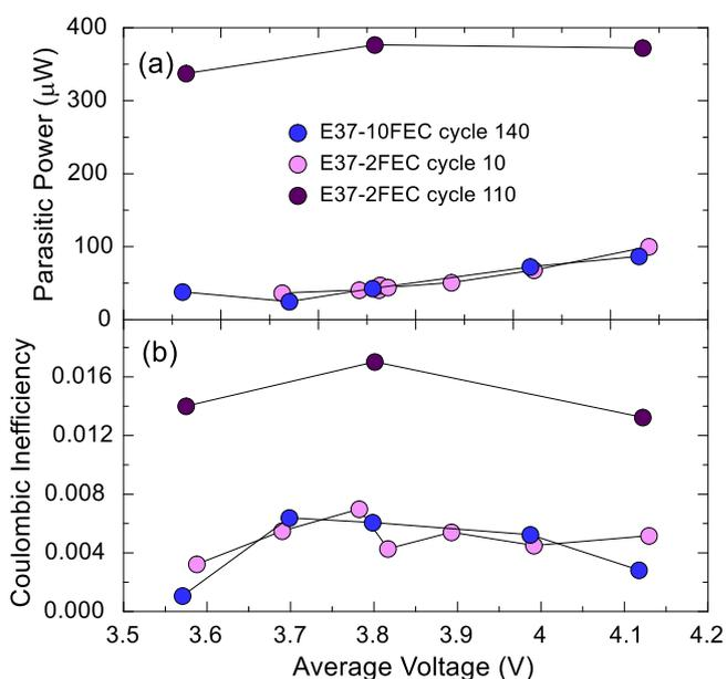
**Figure 10.** (a) Parasitic power and (b) coulombic inefficiency of Gr:Si-alloy//LCO full pouch cells with 3EC:7EMC and 2 wt% FEC or 10 wt% FEC in 1 M LiPF<sub>6</sub> as a function of the average voltage window for various cycle numbers as indicated in the legend.
