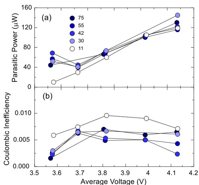
**Figure 4.** (a) Parasitic power and (b) coulombic inefficiency of Gr:Si-alloy//LCO full pouch cells with 23EC:67EMC:10FEC in 1 M LiPF<sub>6</sub> electrolyte as a function of the average voltage window for various cycle numbers as indicated in the legend.
